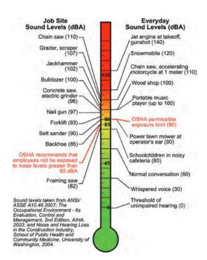
The above chart provides an overview of common sources of workplace noise and their accompanying dBA levels. Source: OSHA.
